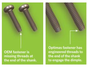
New Fastener: Replaced a trilobular, thread-forming screw (left) with a trilobular, sharp-crested, thread-forming screw (right) to engage the dimple.
