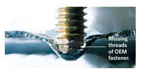
OEM Fastener: A standard trilobular screw can't engage with a dimple pressed into the stamped metal wall of an electrical control box.
