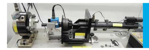
The LabMaster Pro Torque Tensioner used to test fasteners at Optimas' ISO 17025 compliant quality lab in Wood Dale, IL.
