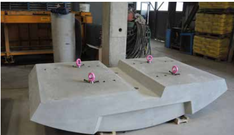
Bolting system used for levelling of pre-cast elements.
